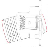
Our product can be easily moved along the horizontal axis. When users position it as desired and release it, the lamp remains fixed in that position. This flexibility perfectly caters to your lighting needs in any environment.
