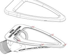
Remove the cap of the product, apply insulation material to the rear side of the product, and secure it with screws at the indicated locations as per the technical drawing.
