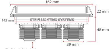
The Driver Is Protected In An Aluminum Housing
