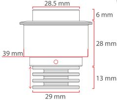
To adjust the indicated part vertically in the drawing you may loosen and tighten the set screws using an Allen wrench.
