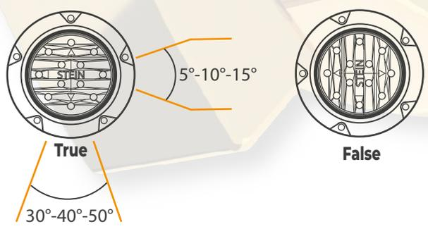
To make the best use of light efficiency the lens angles have been specially optimized to create a parallel light on the sea surface. For example, horizontally at 30°-40°-50° and vertically at 5°-10°-15°, with different angles complementing each other, providing an excellent pattern on the water surface
