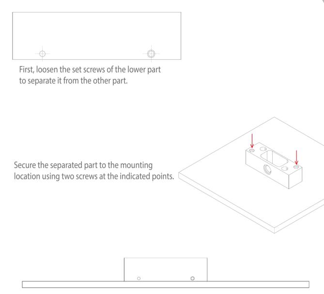
After mounting the part, place the other part back in position and tighten the set screws again.
