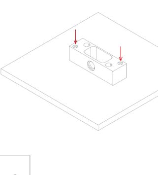
After mounting the part, place the other part back in position and tighten the set screws again.
