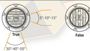
To make the best use of light efficiency the lens angles have been specially optimized to create a parallel light on the sea surface. For example, horizontally at 30°-40°-50° and vertically at 5°-10°-15°, with different angles complementing each other, providing an excellent pattern on the water surface
