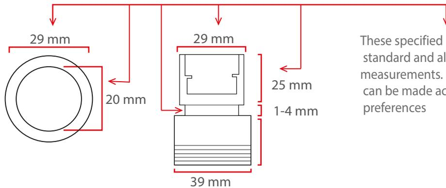
These specified dimensions are standard and also the minimum measurements. Larger dimensions can be made according to your preferences
